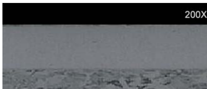
Q2 Artificial Lift Services’ chrome plating: Micro-crack density is so tight that they are not visible. Porosity is well below 15%.
