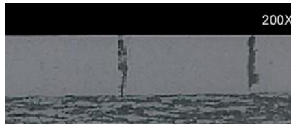
Traditional chrome plating: Macro-cracks in the plating extend thru to the substrate allowing for accelerated corrosion to occur.
