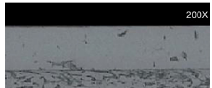
Traditional chrome plating: Large porosity and micro-cracks decrease corrosion resistance.
